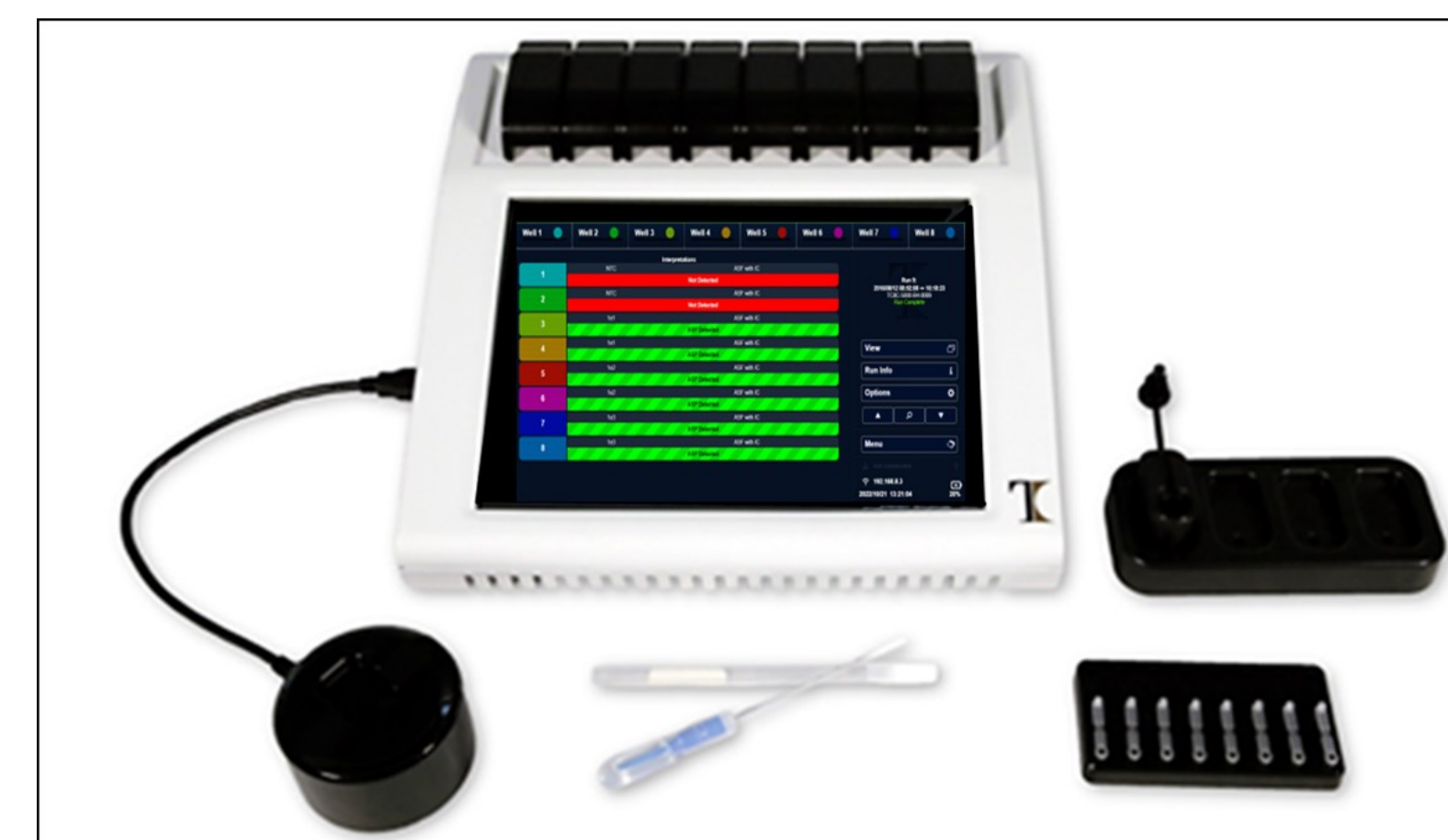
Figure 1. Portable Thermocycler T-COR 8™, with a portable mixer, test cartridge, T-COR 8 tubes, and simple sample collection device.
